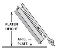
If the platen height is incompatible with the hood type, platen height must be adjusted by an authorized service agent.
